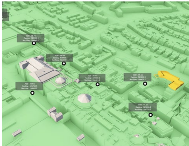
Fig 30 Laser shows how St Nicholas shopping mall is predominantly below the 21m threshold bar some roof elements.
