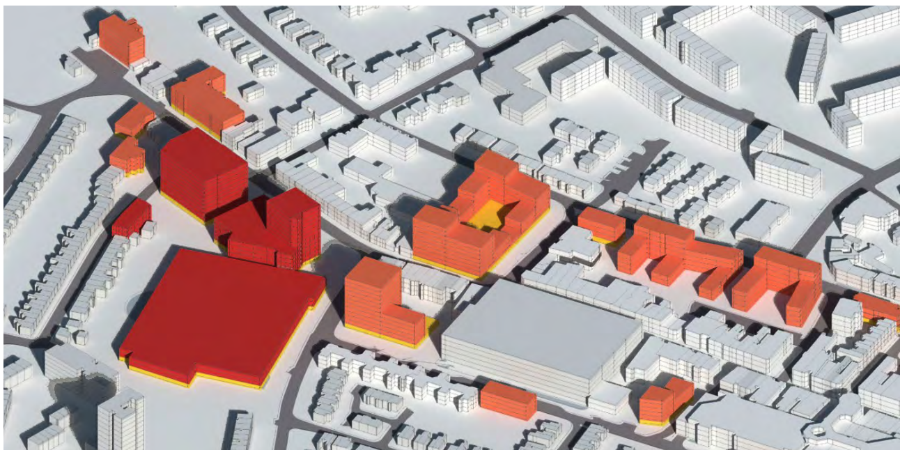
Scale and massing of indicative development proposals within the northern quarter. Red blocks already have planning permission.
